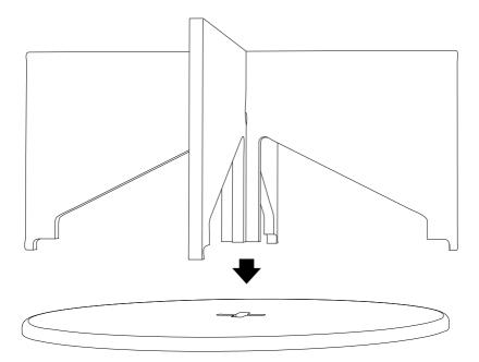
Place top plate on the floor and press legs inside. If needed rotate legs 90  $^{\rm o}$  clockwise until perfect fit!
