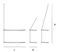
DIMENSIONS L 800 x D 220 x H 1200 mm (long wire) L 31.4 x D 8.6 x H 47.2 " L 800 x D 220 x H 770 mm (short wire) L 31.4 x D 8.6 x H 30.3 "
