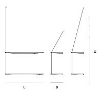
DIMENSIONS L 600 x D 220 x H 1200 mm (long wire) L 23.6 x D 8.6 x H 47.2 " L 600 x D 220 x H 770 mm (short wire) L 23.6 x D 8.6 x H 30.3 "
