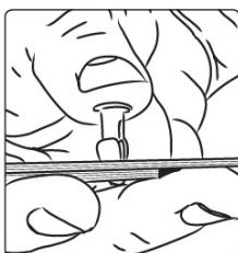
**EN** Take note of the helpful diagram illustrating the importance of supporting the rear of the hole when inserting clips.
