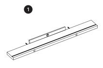
Hold the shelf against the wall, make sure it is leveled. Use the two holes to mark where to drill.
