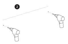
Drill the two holes and insert adequate wall plugs suited for you wall type.
