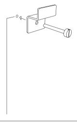
Mount the bracket on the wall. Drill a hole and use a raw plug if necessary, depending on what type of wall it is.
