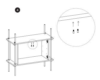
Insert the door stoppers by screwing them into the holes of the top shelf.
