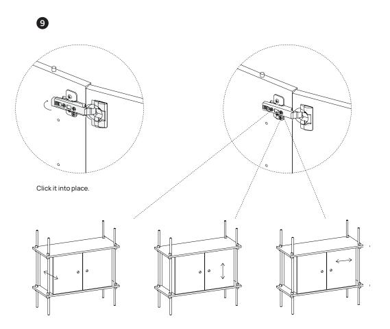
To adjust the placement of the doors, tighten/loosen these three screws.
