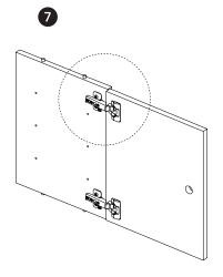
Mount the doors onto the side panels of the cabinet.
