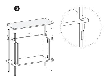
Slide down the top shelf until it sits on the dowels of the side panels. Fasten it with the wedges. Use a hammer to make sure it is secured.
