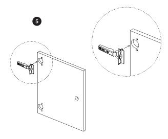
Place the hinges in the large holes of the doors.
