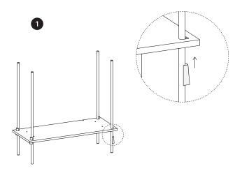
Start by placing the bottom shelf at a desired height, fasten it with the wedges. Use a water level and a hammer to make sure it is leveled and secured.
