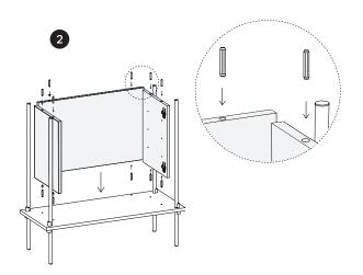
Insert the dowels into the holes of the 'back and side panels. Attach them to the bottom shelf.
