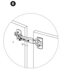
Slide the hinge over the metal plate.
