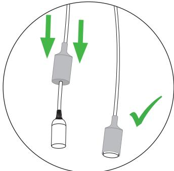
EN - Slide the silicone cover on top the bulb holder
