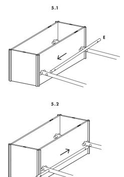
MOUNT THE TWO SMALL DOWELS IN THE RAIL ON EITHER SIDE OF THE LEGS
