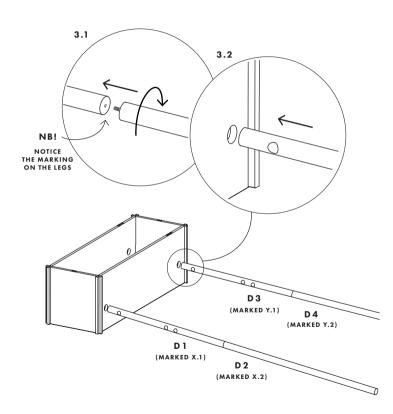
INSERT THE LARGE DOWELS IN THE LEGS UNDER THE TOP AND BOTTOM PLATE. PLEASE NOTE THAT THE DOWELS SHOULD BE HORIZONTAL. IF THIS IS NOT THE CASE, THEN TURN THE LEG 180 DEGREES.
